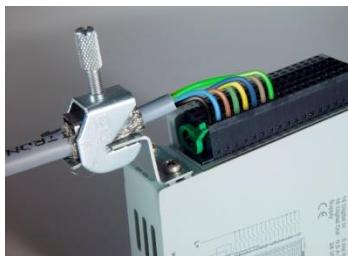
The shield terminal assembly consists of the actual shield terminal, the terminal bracket, two M3x5 screws, 2 washers, and 2 spring washers. Use the 2 screws, washers and spring washers to mount the terminal bracket on the housing mount of the Kuhnke FIO module. Screw the screws into the 2 holes tapped into the bottom of the front side.
